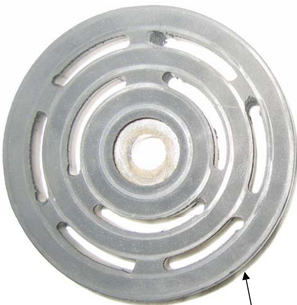
Plate which was in operation. The 6 visible rings mark the sealing plate. As long as these have no infringement, the valve plate still meets specification.
