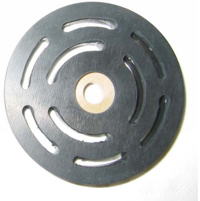
New valve plate which has never been in use. No ring markings can be seen.
